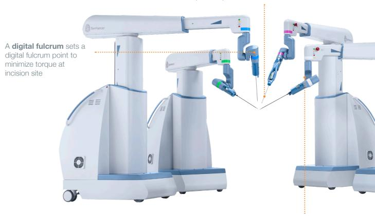
**Open-platform architecture** allows use and integration of existing OR technologies to maximize benefit from capital investments and support surgeon preference Haptic sensing heightens the surgeon's sensing of pressure/ tension through alerts if pressure threshold is reached, for an added layer of security not currently available elsewhere
